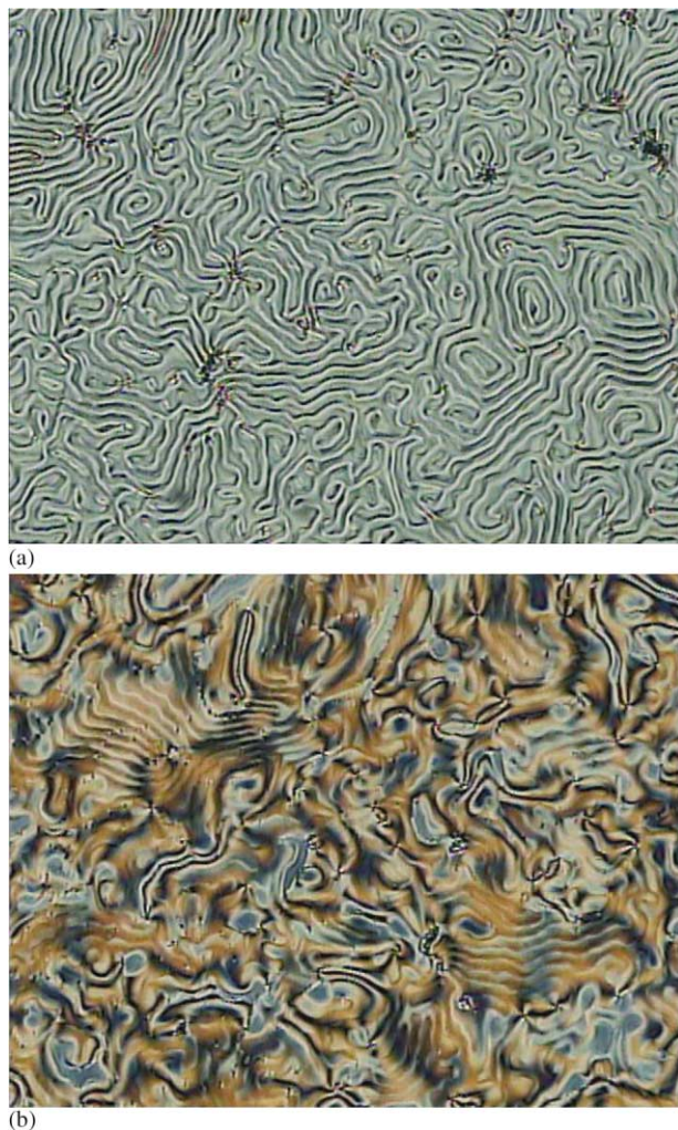
Figure 1. Textures of the chiral phases of binary mixture containing 4 mol% of (+)-2 with the mesomorphic p -decyloxybenzoic acid (a) chiral nematic phase obtained at 135°C on cooling; (b) chiral smectic phase obtained at 112°C on cooling.
